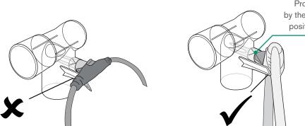
Probe depth is controlled by the tip of the VEE feature positioned against the port
